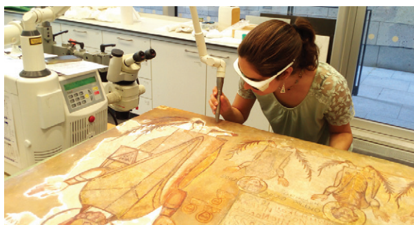
Using an ErYAG laser to remove modern overpaint from a Coptic fresco.
